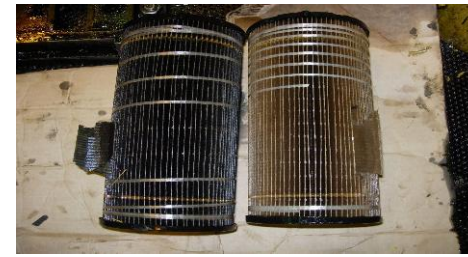
Fuel Filters Before & After Centron 500 hrs of Operation
